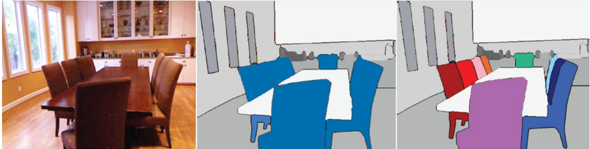
Figure 5.4: Illustration of segmentation of a scene. Left: input image. Middle: semantic segmentation of the scene. All pixels belonging to the class chair are labeled blue. Each instance of the chair class is not distinguished from the others. Right: correct instance segmentation, in which instances are correctly assigned within contiguous segments and across occluded regions. Figure from Silberman et al. (2014).
